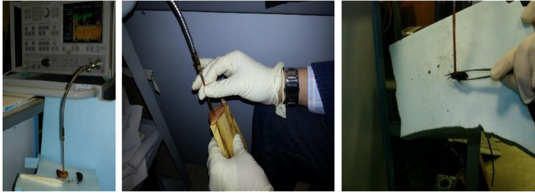
Figure 2. Experimental set up. Left: coaxial cable connected to the Vector Network Analyzer; center: measurement of a wood slice; right: measurement of the adult insect.
