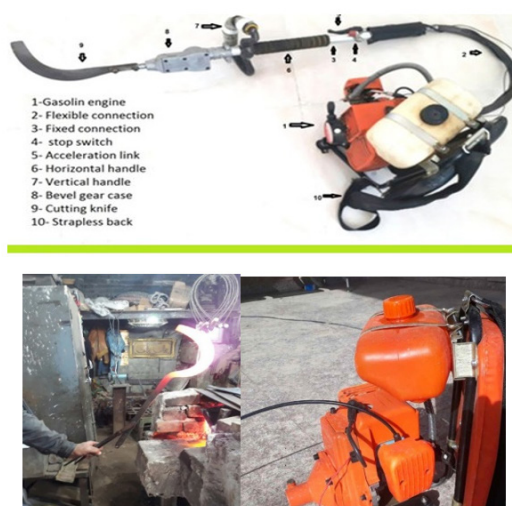
Figure 1. Motorized vibration date palm fronds cutter.
