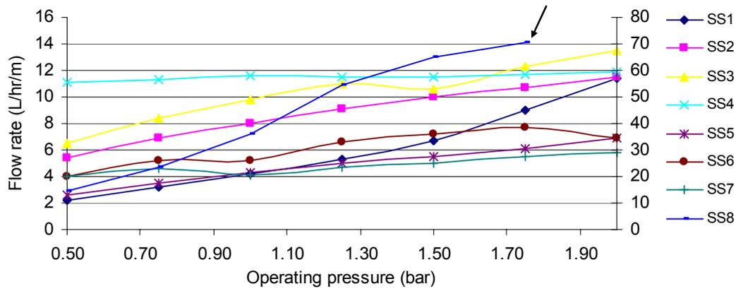
Fig. 3. Curves represent pressure and discharge for subsurface irrigation pipes (the vertical axis of right-special Curve specified arrow).
