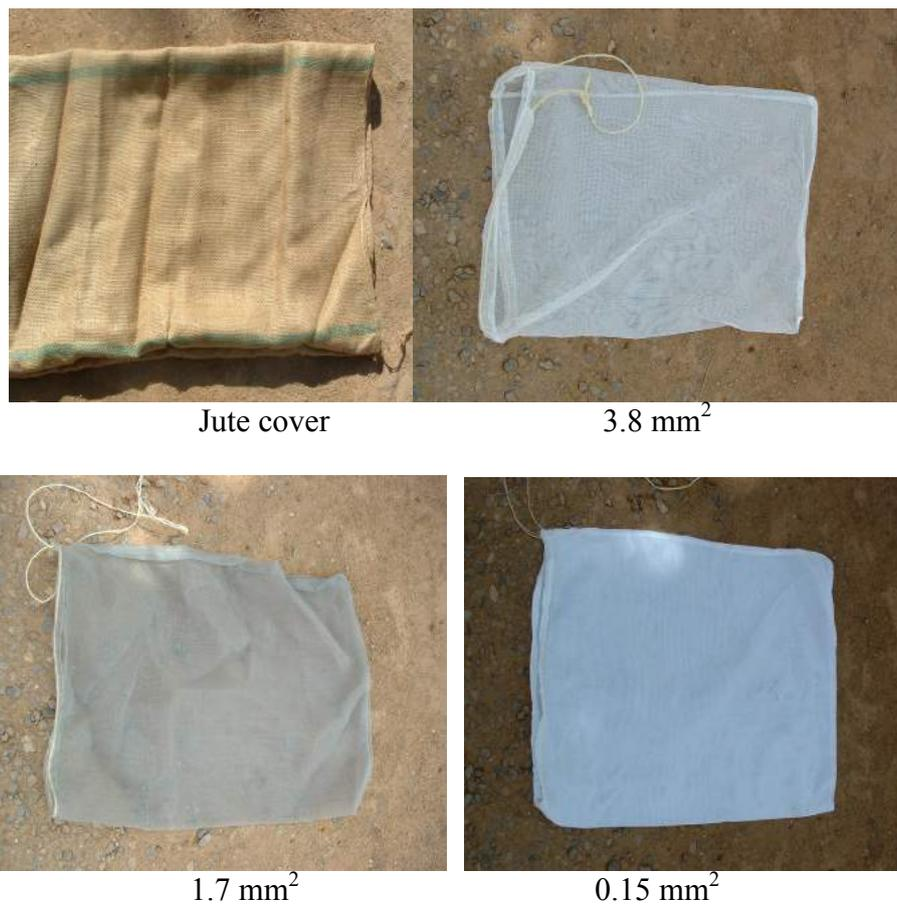
Fig. 3. The four kinds of cover bags used in the experiment.
