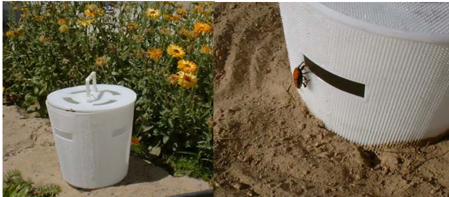
Fig. 15. Rough surface molded plastic R. ferrugineus trap used in the UAE. Trap is used buried in ground to level of entry ports.
